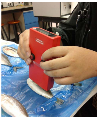
Fig. 4: Appropriate way to measure using Torrymeter
